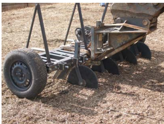
Picture 26 aeration tubing plow (source: Scott D. Wallace)
