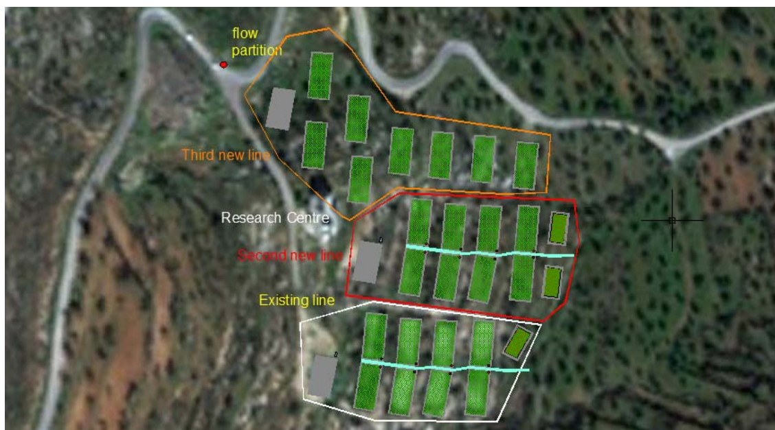
Picture 21 Increase the capacity of the existing treatment adding other similar parallel lines
