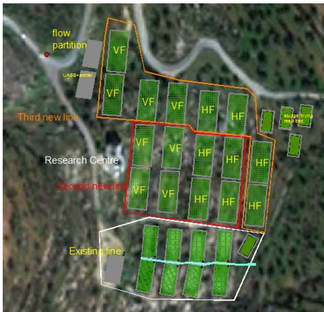
Picture 23 Increase the capacity of the existing treatment adding other lines with the combination of vertical and horizontal flow systems
