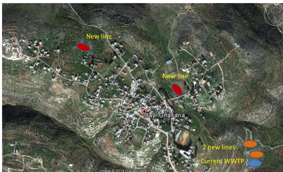
Picture 22 Possible locations for other decentralized system to cover totally the wastewater treatment demand
