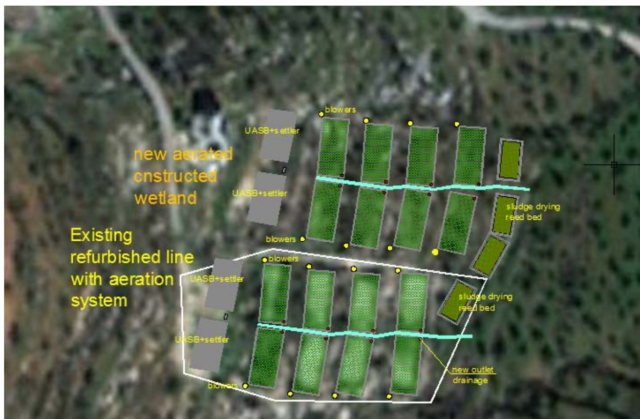
Picture 27 Upgrade the capacity of the existing treatment with forced aeration technology.
