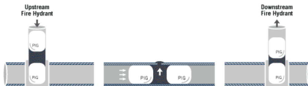
Figure 4 Representation of the curapipe technology application (picture taken from the Leakcure project www.curapipe.com )
