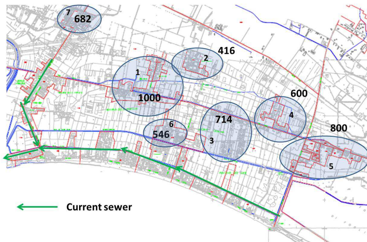
Picture 15 Existing sewer network of Borgo Sabotino and unconnected settlements
